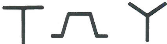
FIG. 1 Typical Cross Sections of Line Post Types
