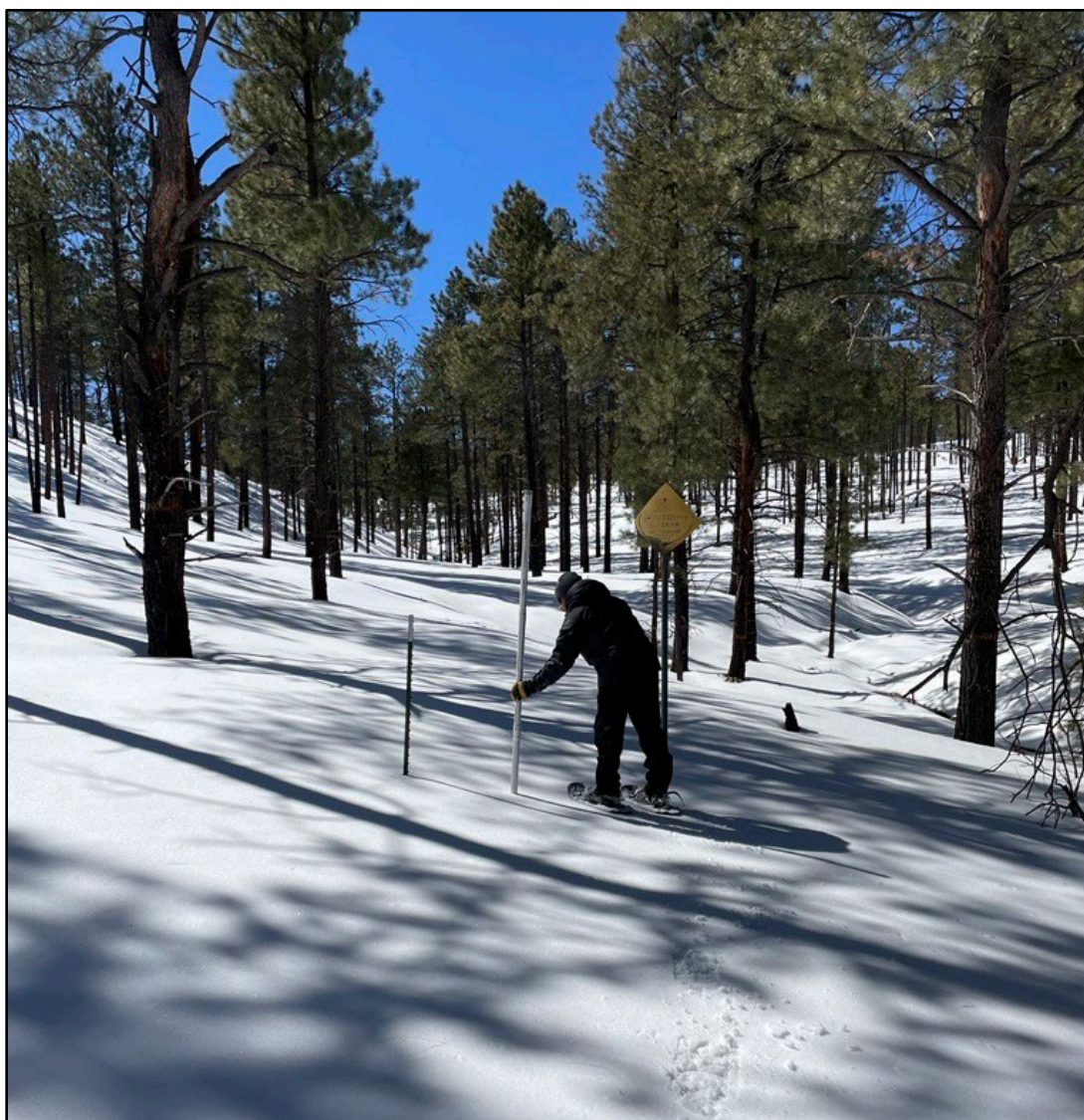
Logan Peterson, NRCS Soil Scientist, performs a measurement at the Ojo Redondo manual snow course in the Zuni Mountains on February 28 th , 2023. Snow Water Equivalent [SWE] at this site measured 192% of normal on this visit. NRCS Photo: Jaz Ammon
